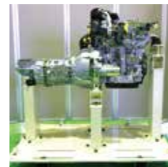
Set up jigs for bench tests
